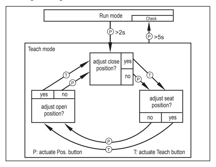
After installation you have to adjust the unit to the valve positions to be detected.
