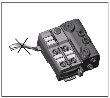
Take care in laying the AS-i flat cable, the flat cable should be laid straight for about 15 cm.
