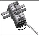
Take care in laying the AS-i flat cable, it should be laid straight for about 15 cm.
