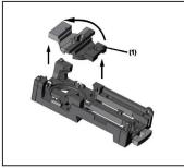
The supplied lower part the flat cable can be aligned in three directions.
