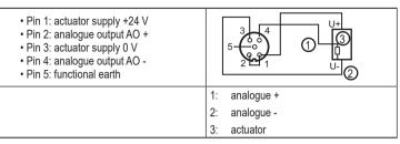
Wiring diagram of a 3-wire actuator without own supply, actuator load connected to U+.
