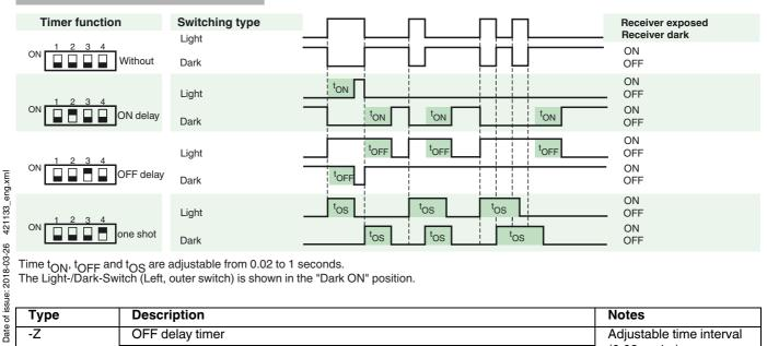
Time  $t_{ON}$ ,  $t_{OFF}$  and  $t_{OS}$  are adjustable from 0.02 to 1 seconds. The Light-/Dark-Switch (Left, outer switch) is shown in the "Dark ON" position.
