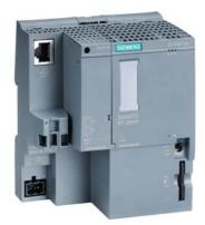
\*\*\* spare part \*\*\* SIMATIC DP, CPU 1510SP-1 PN for ET 200SP, central processing unit with work memory 100 KB for program and 750 KB for data, 1st interface: PROFINET IRT with 3-port switch, 72 ns bit performance, SIMATIC Memory Card required, BusAdapter required for port 1 and 2
