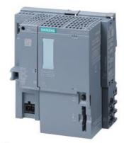
SIMATIC DP, CPU 1512SP-1 PN for ET 200SP, central processing unit with work memory 400 KB for program and 2 MB for data, 1st interface: PROFINET IRT with 3-port switch, 25 ns bit performance, SIMATIC Memory Card required, BusAdapter required for port 1 and 2
