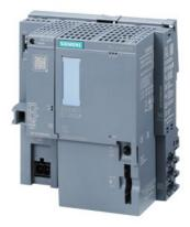
SIMATIC DP, CPU 1510SP-1 PN for ET 200SP, central processing unit with work memory 200 KB for program and 1 MB for data, 1st interface: PROFINET IRT with 3-port switch, 25 ns bit performance, SIMATIC Memory Card required, BusAdapter required for port 1 and 2
