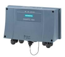
SIMATIC HMI connection box Advanced for Mobile Panels, wall mounting, PROFINET and PROFIsafe, connection of safety relay, emergency stop circuit bridging, terminal detection, Integrated switch, MRP client, IRT
