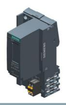
SIMATIC ET 200SP, PROFINET, 2-port interface module IM 155-6PN/2 High Feature, 1 slot for BusAdapter, max. 64 I/O modules and 16 ET 200AL modules, S2 redundancy, multi-hotswap, 0.25 ms, isochronous mode, optional PN strain relief, including server module
