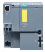
SIPLUS ET 200SP CPU 1510SP F-1 PN T1 rail based on 6ES7510-1SJ01-0AB0 with conformal coating, -25...+60 °C, OT1 with ST1/2 (+70 °C für 10 minutes), central processing unit with work memory 150 KB for program and 750 KB for data, 1st interface, PROFINET IRT with 3-port switch, 72 ns bit performance, SIMATIC Memory Card required, BusAdapter required for port 1 and 2
