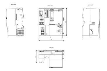
The Siemens SIMATIC DP, CPU 1514SP F-2 PN for ET 200SP, central processing unit with work memory 900KB for program and 3.5 MB for data, 1st interface PROFINET IRT with 2-port switch, 2nd interface PROFINET RT, 6 ns bit performance.
