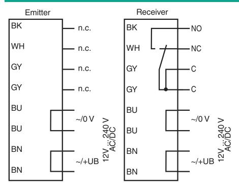
The relay-functions "NC" and "NO" bear on the switching mode "Dark-ON".
