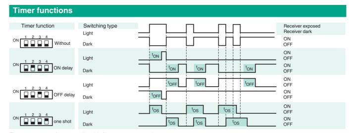
Time  $t_{ON}$ ,  $t_{OFF}$  and  $t_{OS}$  are adjustable from 0.1 to 10 seconds. The Light-/Dark-Switch (Left, outer switch) is shown in the "Dark ON" position.
