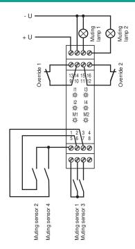
This module can only be operated within an evaluation device of the SafeBox SB4 type.
