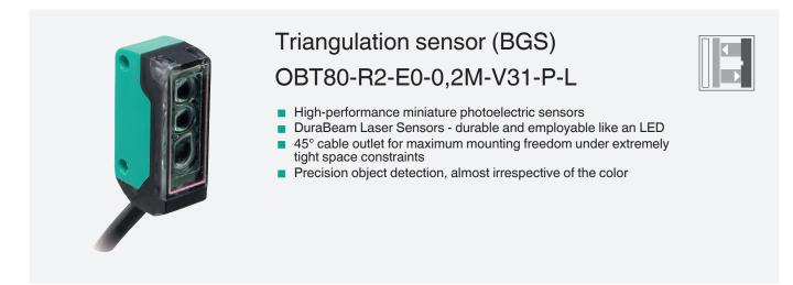
Laser triangulation sensor with background suppression, ultra-small design with M2 mounting, 80 mm sensing range, light on, NPN output, 200 mm fixed cable with plug M8, 4-pin
