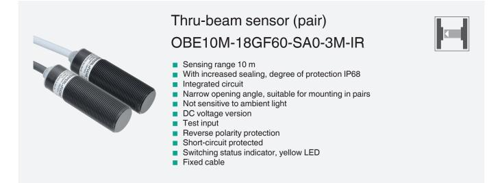
Thru-beam sensor, M18 threaded housing design, plastic housing, 10 m detection range, infrared light, light/dark on, DC version, 2 NPN outputs, fixed cable
