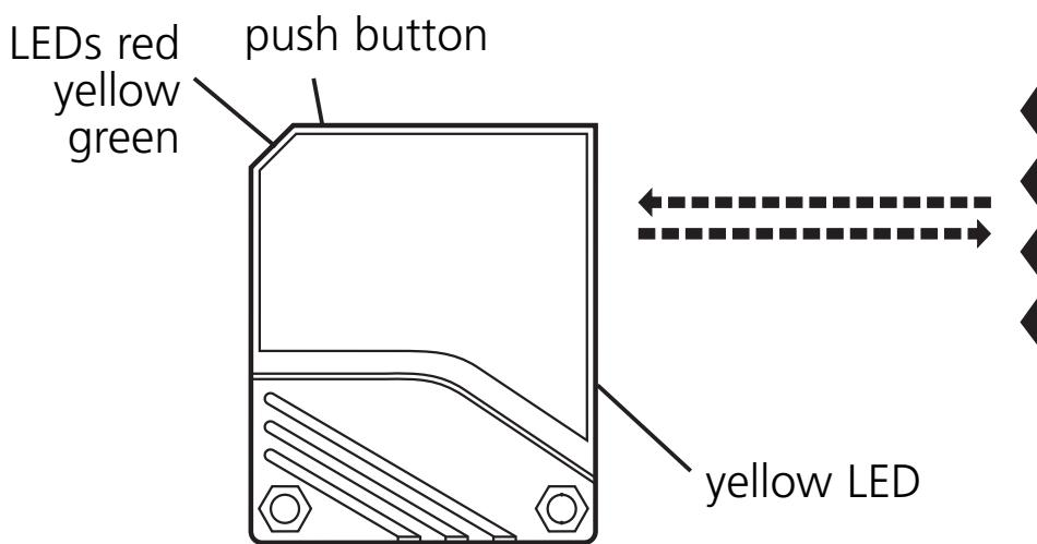
Fix prismatic reflector / reflective tape in desired position. Align the photocell photocell towards the reflector and fasten it to a mounting bracket; the light spot must hit the prismatic reflector.
