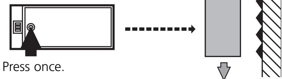
The yellow and green LEDs go out for approx. 1s, after approx. 3s the green LED is on.
