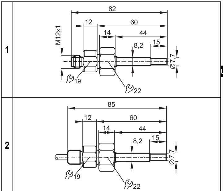
Dimensions are in millimeters
