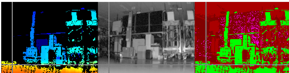
Fig. 12: Distance image (left), amplitude image (centre) and confidence image (right)
